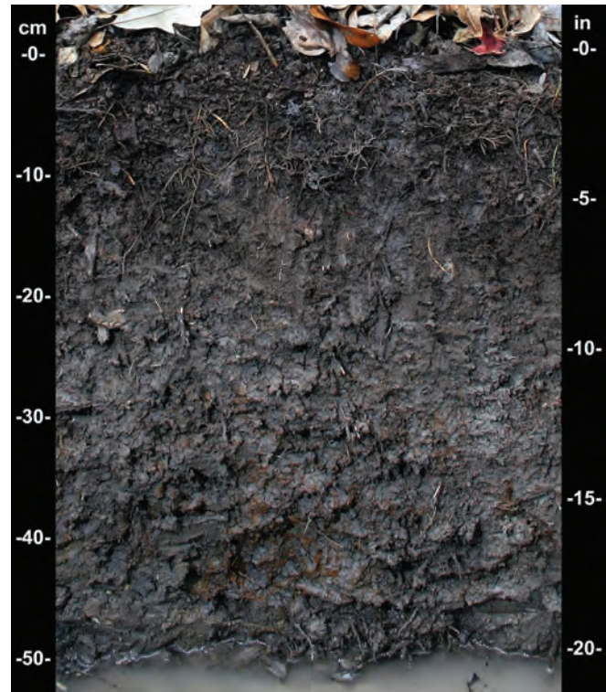
Figure 52.—The gleyed matrix in this soil starts at a depth of about 15 cm. The matrix color has value of 4 or more and is shown on one of the pages showing gleyed colors in the “Munsell Soil Color Book” (X-Rite, 2009).
