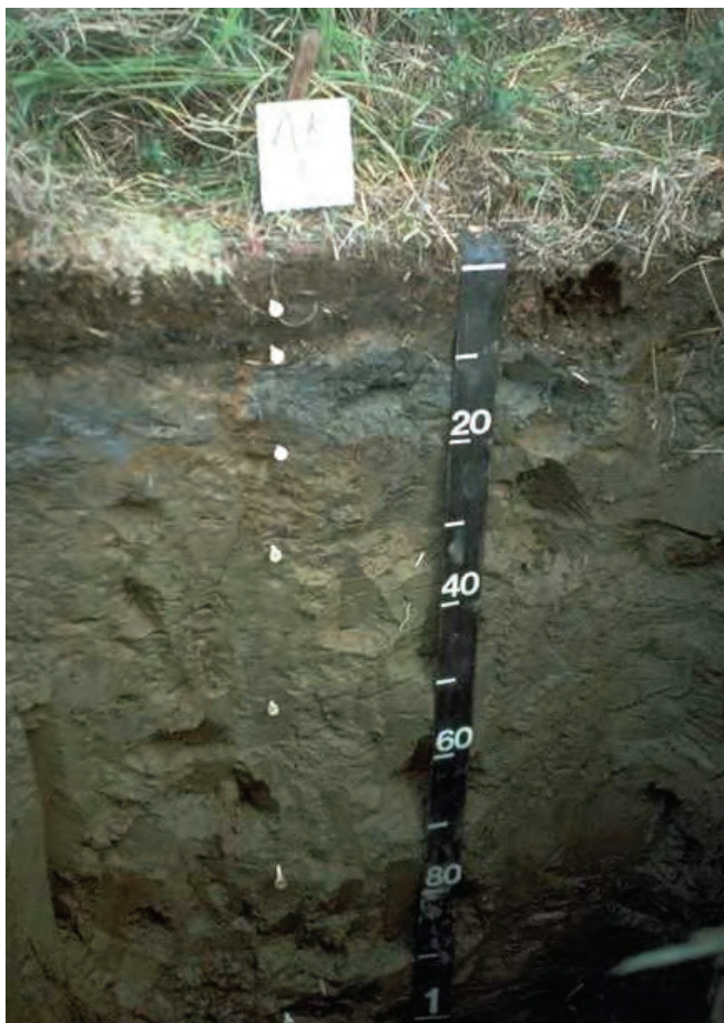
Figure 18.—Indicator A13, Alaska Gleyed. The bluish band at a depth of about 20 cm indicates the presence of reduced soil material. The material below 20 cm reflects both the color of the parent material and soil weathering under aerobic conditions.
