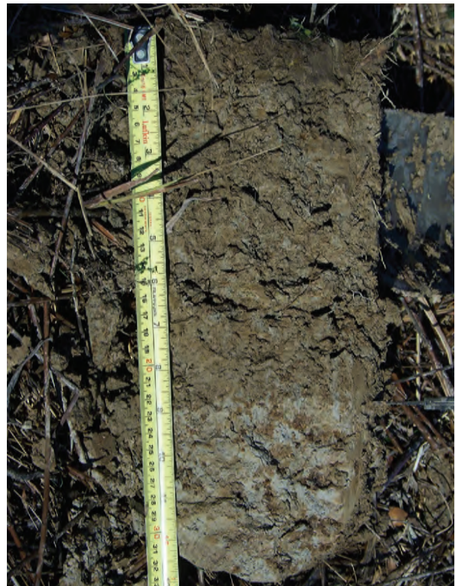
Figure 4.—The lower portion of this soil profile meets the color and depth requirements of indicator F3, Depleted Matrix; however, the upper portion of the profile contains a layer with chroma of more than 2 that is more than 15 cm (6 inches) thick. As a result, the requirements of indicator F3, Depleted Matrix, are not met.
