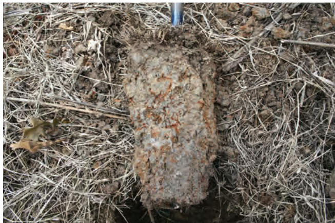
Figure 46.—A depleted matrix with value of 4 or more and chroma of 2 or less. Redox concentrations occur as soft masses and pore linings.
