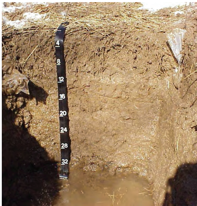
Figure 42.—Indicator F3, Depleted Matrix, in red parent material. If a soil that formed in red parent material stays wet and anaerobic long enough, it may develop the indicator F3.
